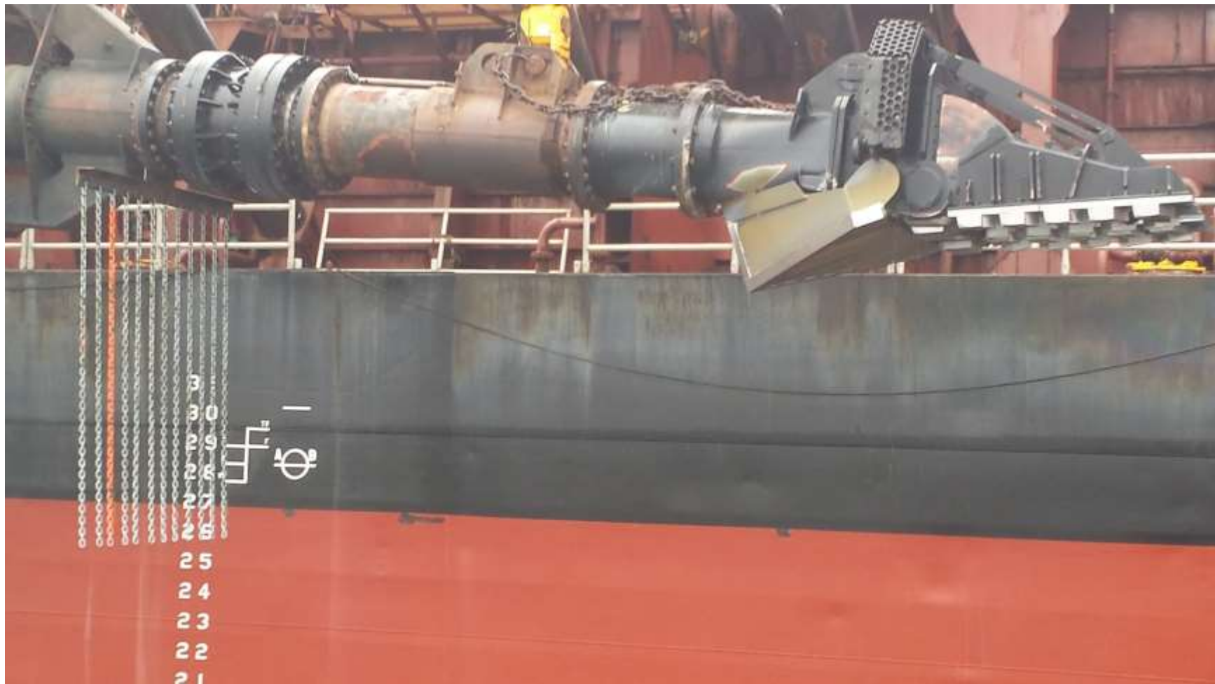
Figure 2-5 Essayons with Recently Fabricated Dragarm Tickler Chains and Draghead Turtle Deflector.
