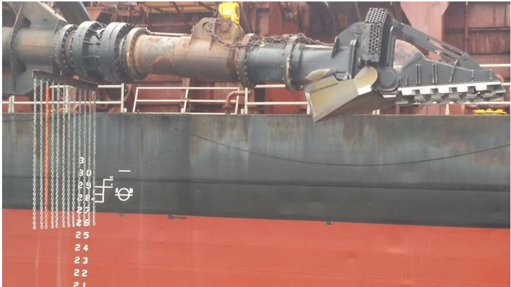
Figure 2-5 Essayons with Recently Fabricated Dragarm Tickler Chains and Draghead Turtle Deflector
