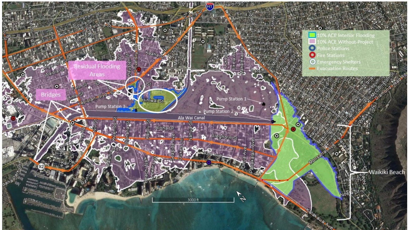
Figure 23. Potential Flooding Areas Due to Failure of Interior Drainage Systems or Residual Interior Flooding
