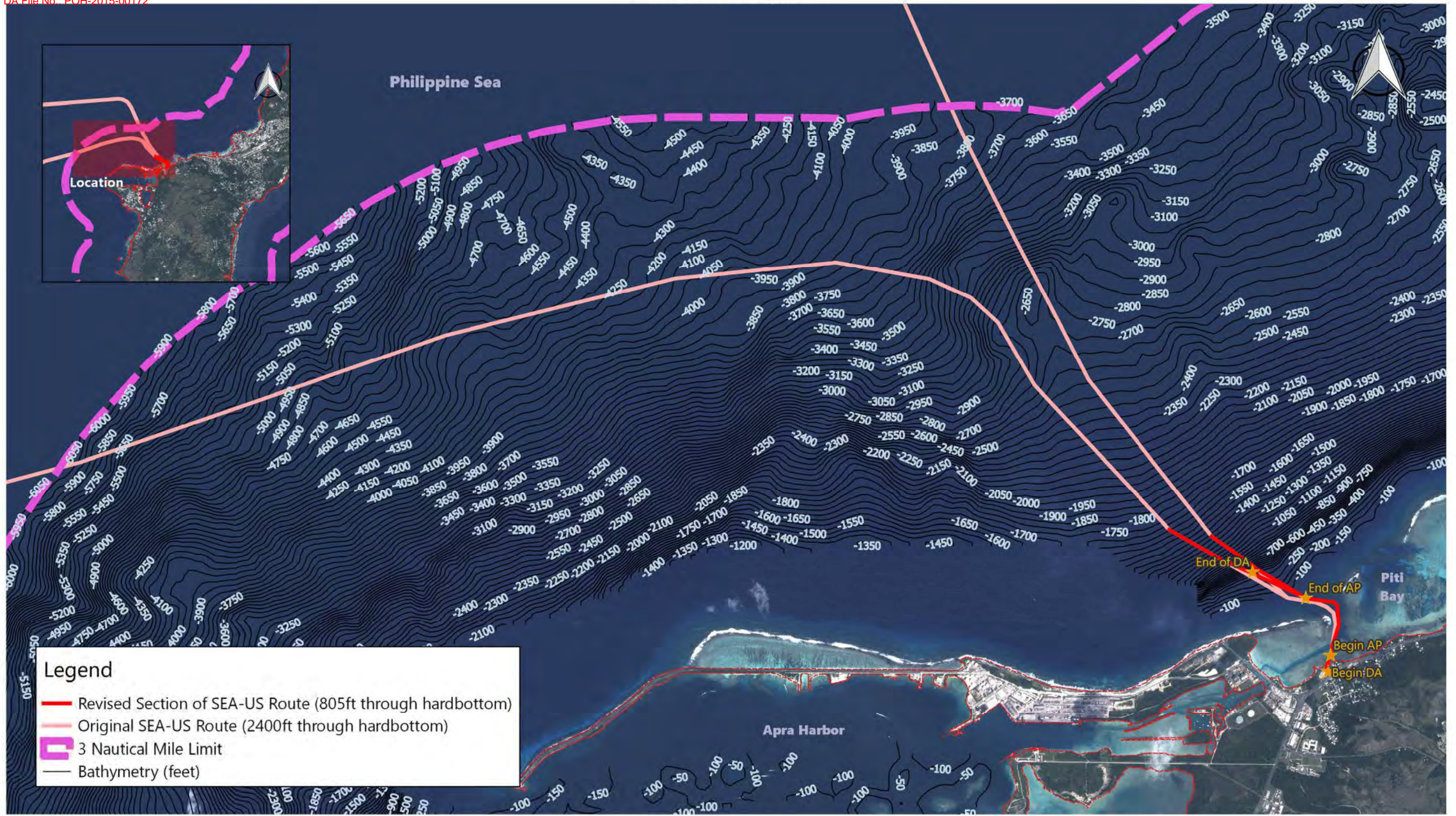
New SEA-US Cable Route from Piti Landing Site Out to Three Nautical Miles
