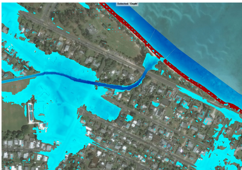
Figure 6-19: Resulting Impact from High Sea Level Change (Red) in 2125 for the 1% AEP Flood Profile for Unnamed Stream #1, Kaiona Watershed
