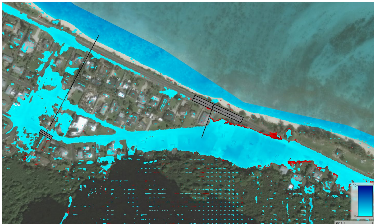
Figure 6-15: Resulting difference in the 1% AEP floodplain boundary due to operational (cleared) culverts in Eastern Waimānalo
