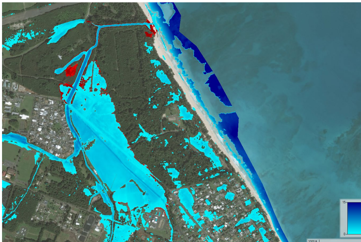
Figure 6-14: Resulting difference in the 1% AEP floodplain boundary between the original, existing conditions model (red) and dredged scenario (blue) for Puha (Inoaole) Stream
