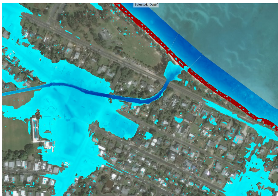
Figure 2-27: Resulting Impact from High Sea Level Change (Red) in 2125 for the 1% AEP Flood Profile for Unnamed Stream #1, Kaiona Watershed
