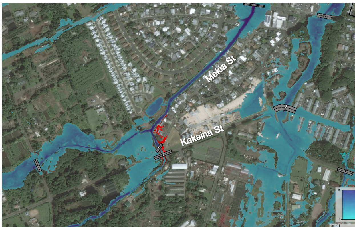
Figure 2-19: Increased flooding due to culvert obstructions near Mekia St
