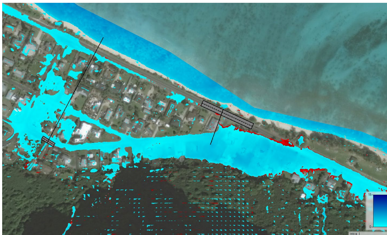
Figure 2-22: Resulting difference in the 1% AEP floodplain boundary due to operational (cleared) culverts in Eastern Waimānalo
