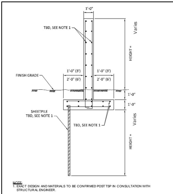
**Figure 2-3. Typical Floodwall Section**
