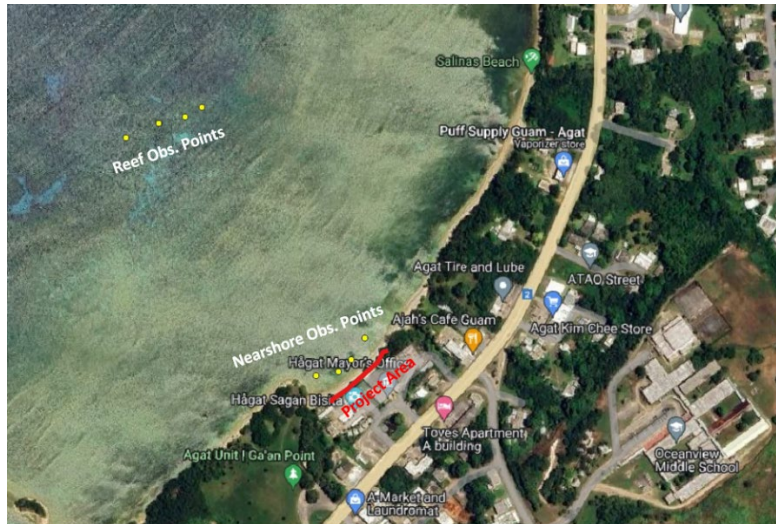
Figure 15. Locations of the two observation-point transects for wave height ( H_s ) outputs from STWAVE
