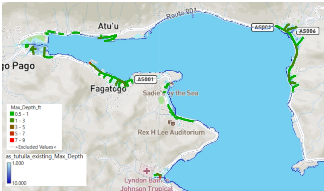
Figure 3-12: Map of Existing Scenario inundation hazard on roads near Pago Pago on the island of Tutuila under the existing NOAA MEOW Storm Surge event at Pago Pago, further showing the vulnerability of Route 1. Source: USACE, 2021
