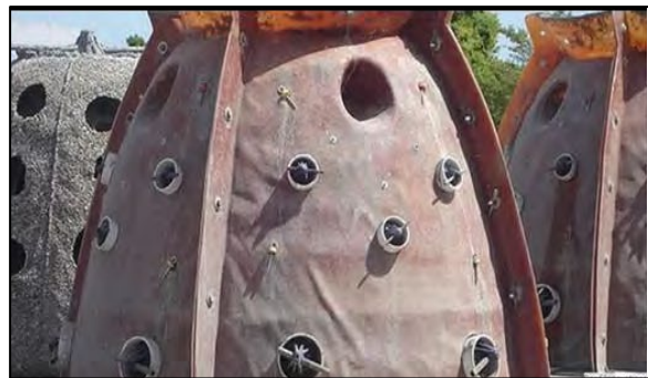
Fiberglass Reef Ball molds (example).
