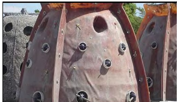
Fiberglass Reef Ball molds (example).
