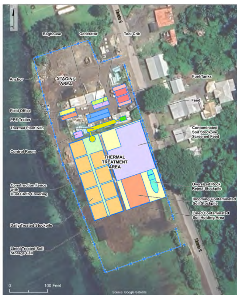
Figure 4. Thermal Treatment and Staging Area Layout
