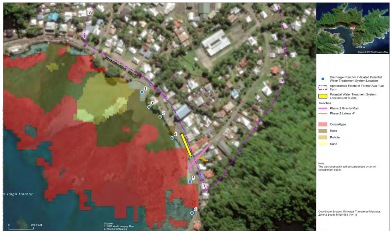
Figure 2. Aua Village map showing the possible locations of the discharge pipe (1-6), the wastewater treatment plant, and sewer installation work.
