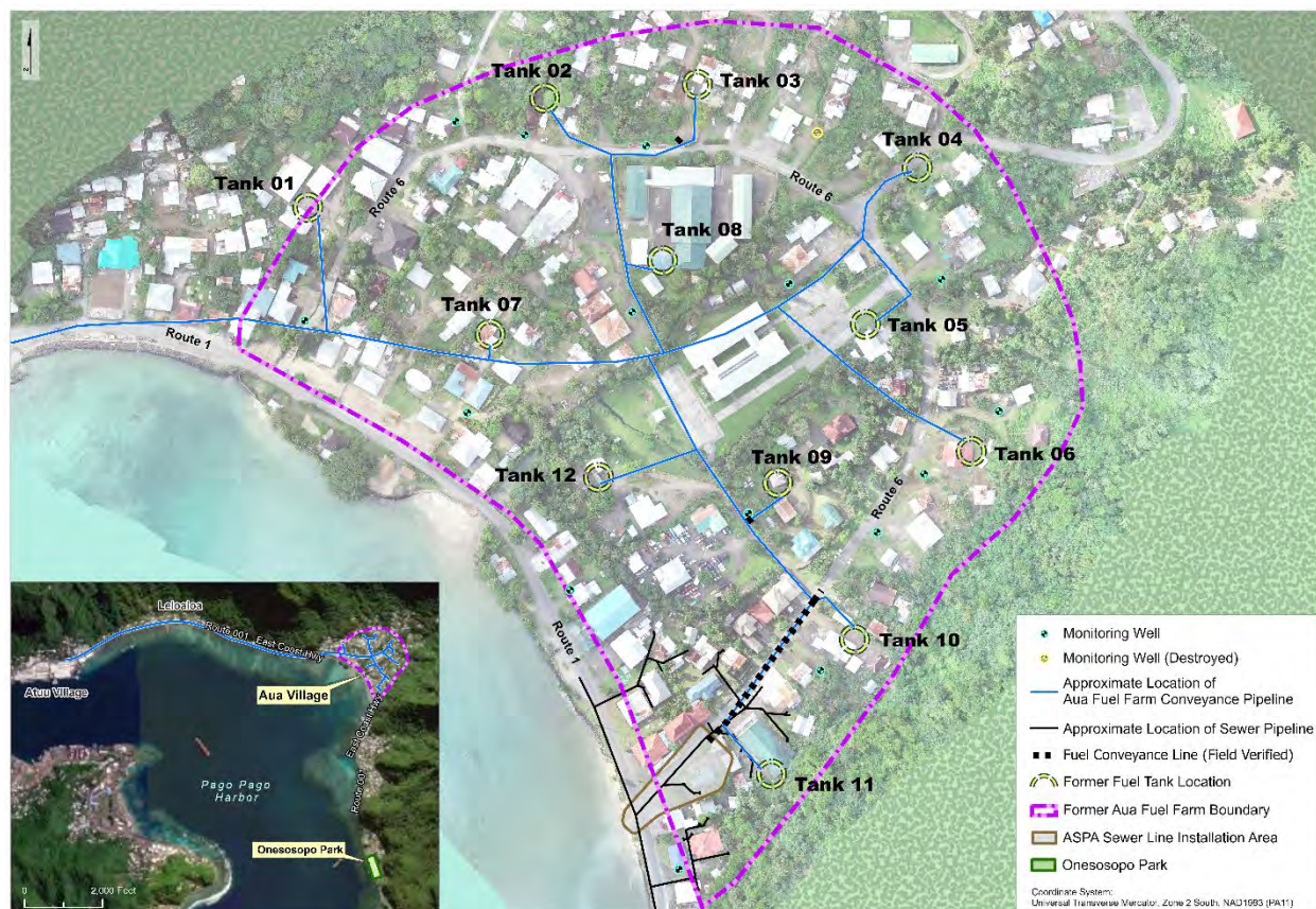
Figure 2. Former Aua Fuel Farm Pipeline Network
