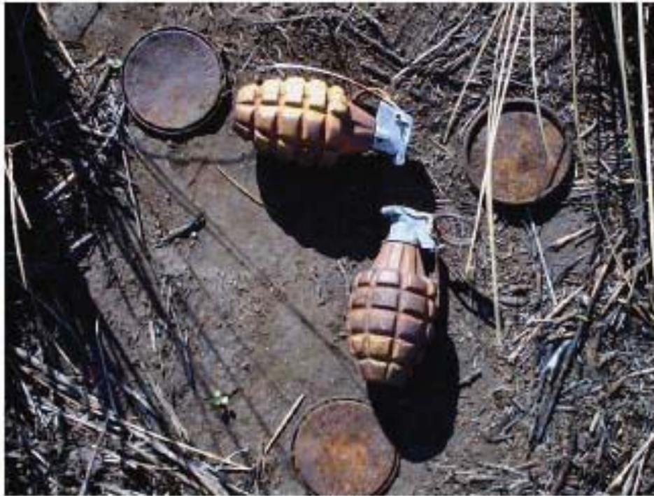
Weight is 1.4 lbs Filler is 1.75 oz of TNT Fuze delay is 4 to 5 seconds
