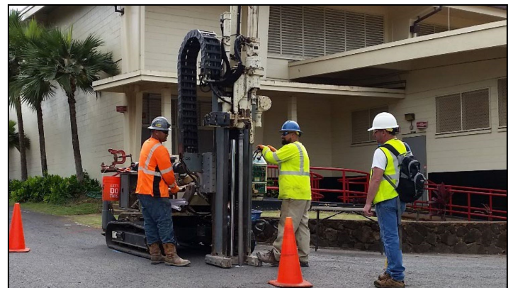
Photo 1: Sample collection using direct push drill rig at Radford High School
