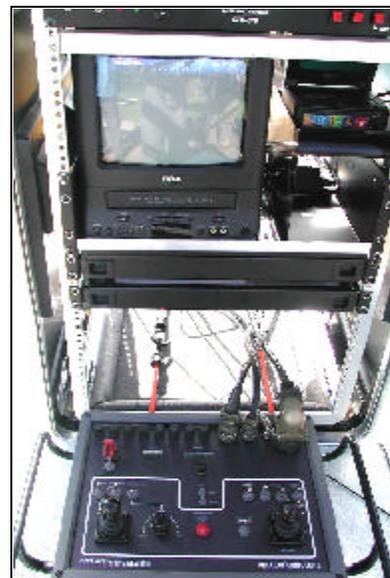
In addition to basic speed, direction and depth controls for the ROV (Remote Operation Vehicle), instrumentation also includes a television, a video cassette tape recorder and a digital recorder for collecting and recording Global Positioning location plots and visual information in both digital and VHS formats.
