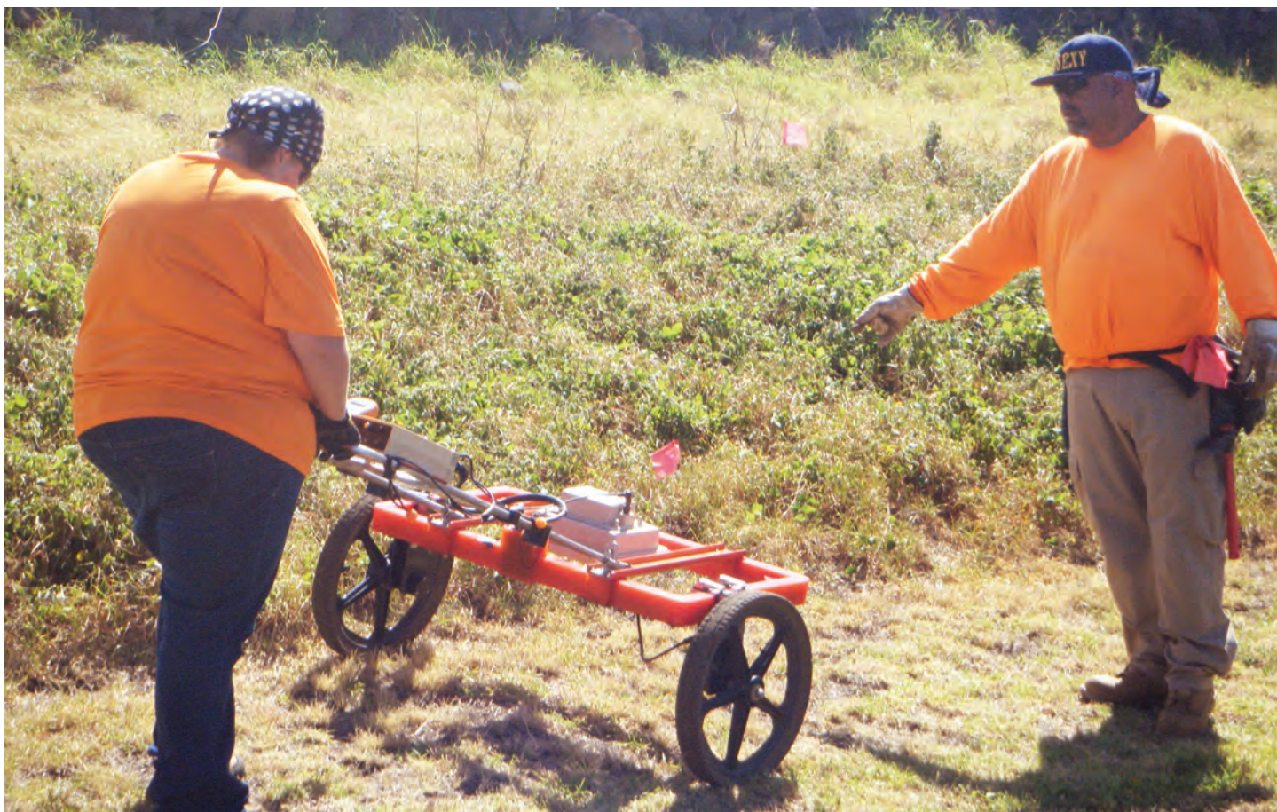
Waikoloa FUDS contract workers from Environet, Inc. use a ground penetrating radar to re-acquire and search for unexploded ordnance anomalies on the first day of a three-day ordnance investigation inside the Sandalwood Subdivision near Waimea on the island of Hawaii Photos by Dino W. Buchanan
