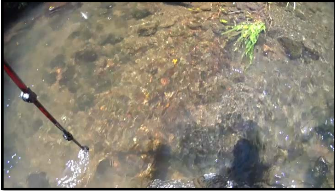
Figure 77: Sub-optimal Embeddedness class. The larger cobbles are surrounded between 25% and 50% by fine or sand substrates.
