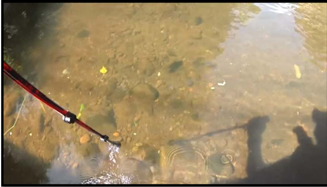
Figure 79: Poor Embeddedness class. Most boulders are surrounded by greater than 75% by fine substrate.
