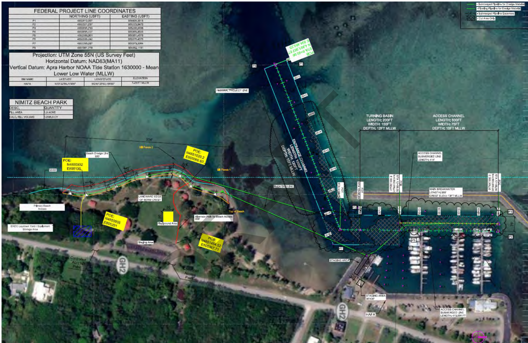
Figure 6 Site Plan - Proposed Action and Action Area, Agat SBH and Nimitz Beach Park (ERDC 2025) Maintenance dredging footprint to right (cross hatch gray polygon), dredged material conveyance pipeline (green line), beach reclamation fill footprint to left (red outline polygon)
