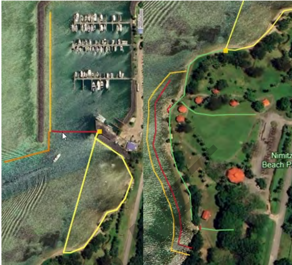
Figure 12 Dredged Material Pipeline Conveyance Alternate alignments are presented. Pipeline from entrance channel (dark orange) and Access Channel (light orange) in harbor will feed to submerged pipeline (red) and to harbor booster pump (light orange square) and convey material to floating pipeline (yellow) that will either cross the corridor and land on Nimitz Beach or follow the beach crest of the shoreline. Pipeline on shore will follow beach contour to beach reclamation fill area (green). Access Ingress/Egress path at Nimitz Beach Park in green with preferred alignment to south and contingency alignment to north. Beach reclamation fill area seaward limit (red) and approximate stabilized toe at end of project (light orange).
