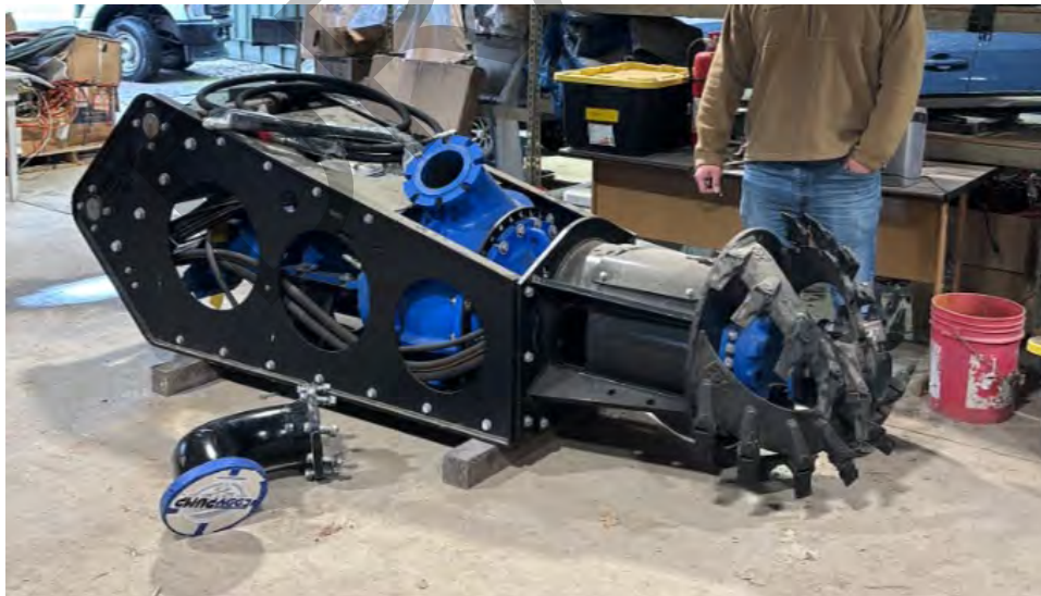
Figure 11 Dredge Head to be Attached to Long Reach Excavator
