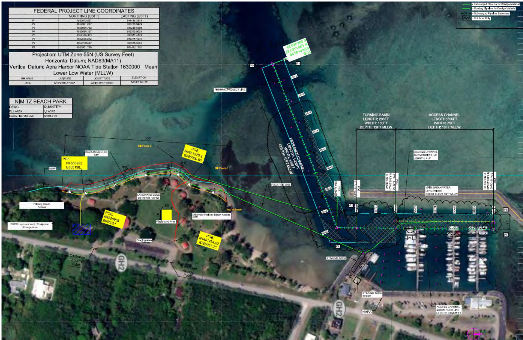
Figure 1 Site Plan - Proposed Action and Action Area, Agat SBH and Nimitz Beach Park (ERDC 2025) Maintenance dredging footprint to right (cross hatch gray polygon), dredged material conveyance pipeline (green line), beach reclamation fill footprint to left (red outline polygon)
