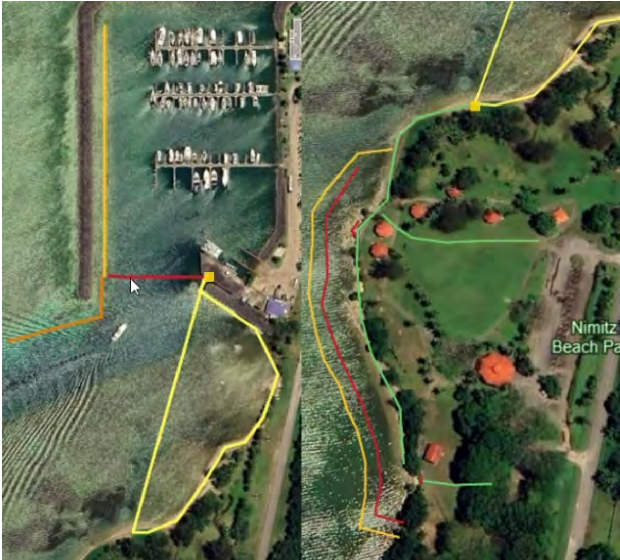
Figure 6 Dredged Material Pipeline Conveyance Alternate alignments are presented. Pipeline from entrance channel (dark orange) and Access Channel (light orange) in harbor will feed to submerged pipeline (red) and to harbor booster pump (light orange square) and convey material to floating pipeline (yellow) that will either cross the corridor and land on Nimitz Beach or follow the beach crest of the shoreline. Pipeline on shore will follow beach contour to beach reclamation fill area (green). Access Ingress/Egress path at Nimitz Beach Park in green with preferred alignment to south and contingency alignment to north. Beach reclamation fill area seaward limit (red) and approximate stabilized toe at end of project (light orange).
