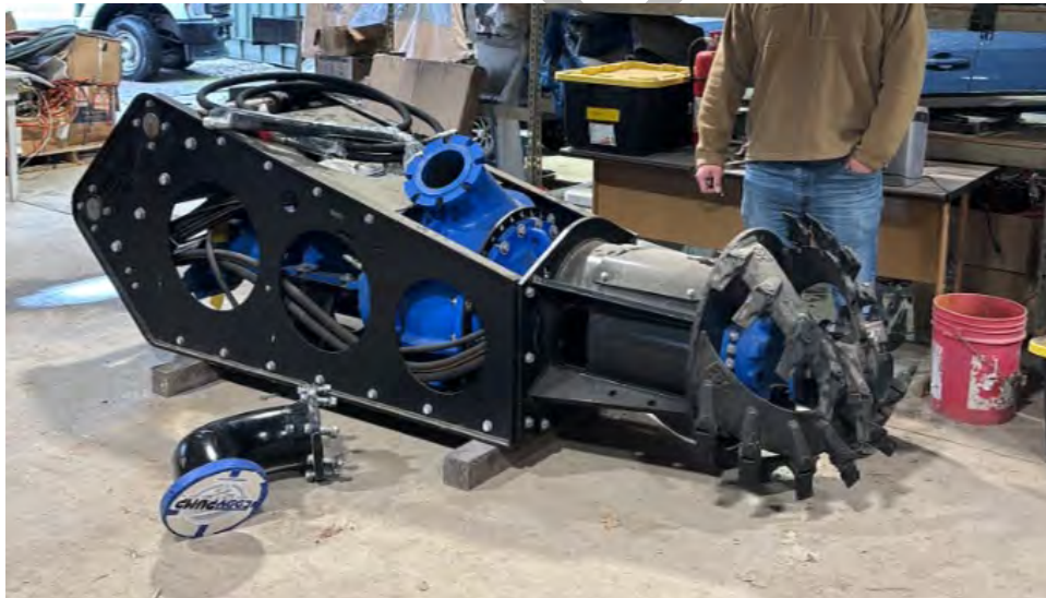
Figure 5 Dredge Head to be Attached to Long Reach Excavator
