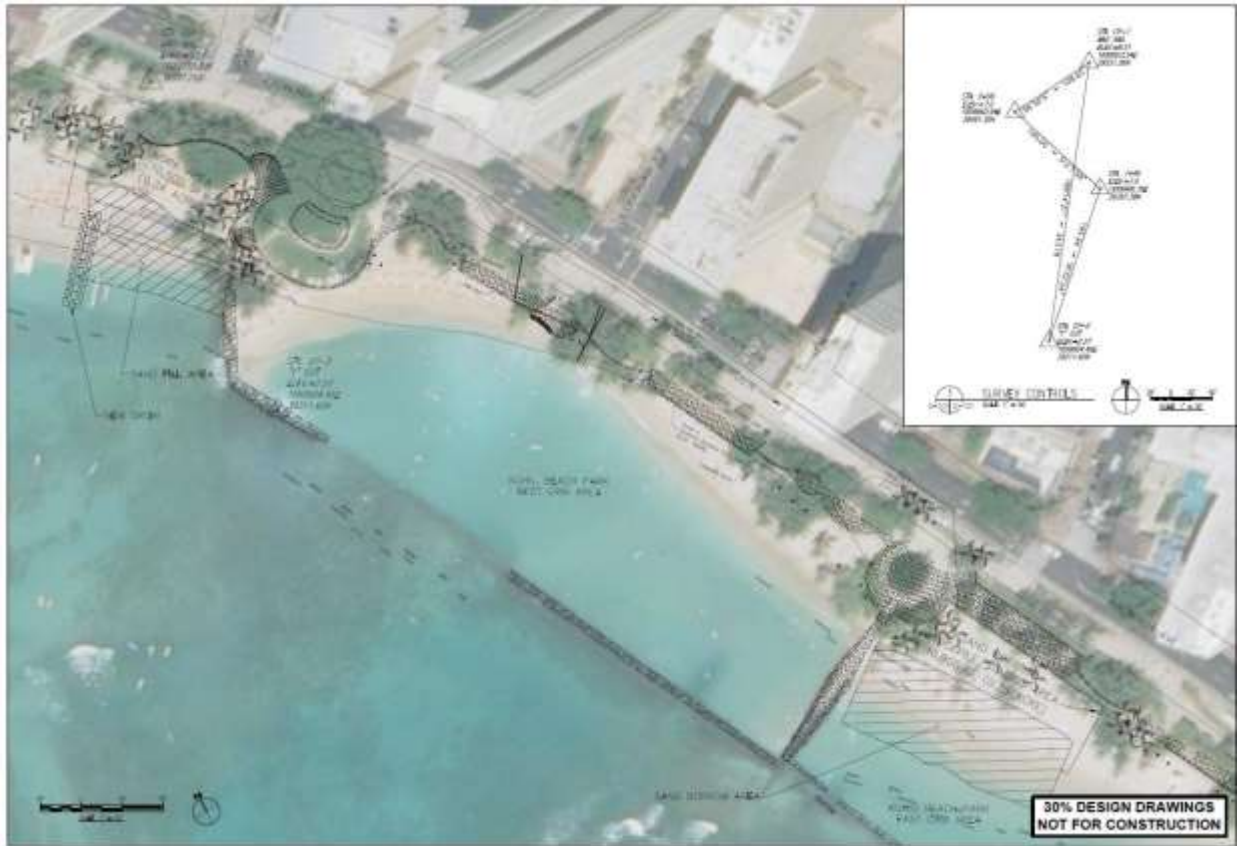
Attachment – Figure 2 General Plan Showing Sand Borrow and Disposal Sites DA File No. POH-2018-00220
