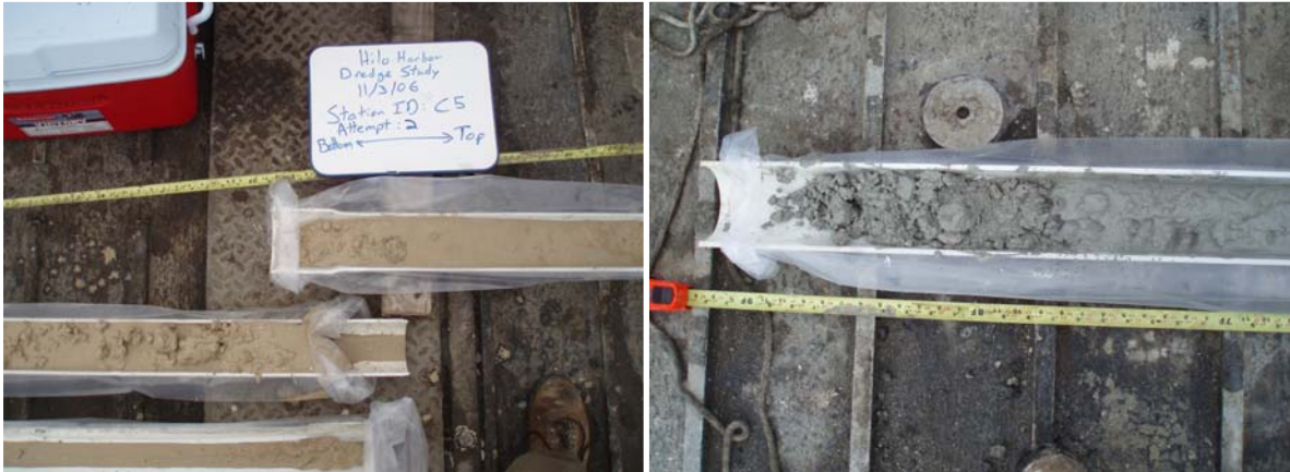
Figure 9. View of typical core, laid out in sampling trays. Coral detritus in sand matrix (left). Coral detritus in a silt/sand/basalt matrix (right).
