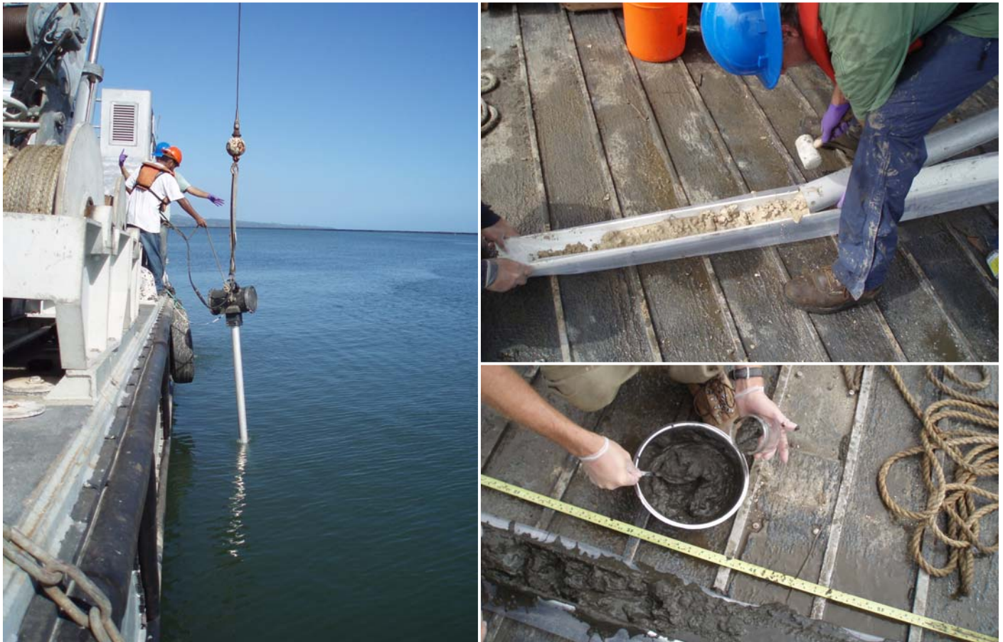
Figure 5. Sampling activities. Left: Positioning of vibracoring equipment. Upper-right: Extraction of the core contents into lined sampling tray. Bottom-right: Sub-sampling the core contents, homogenization, filling sample jars.
