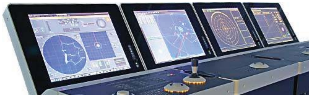
Kongsberg Maritime commercially available Dynamic Positioning System
