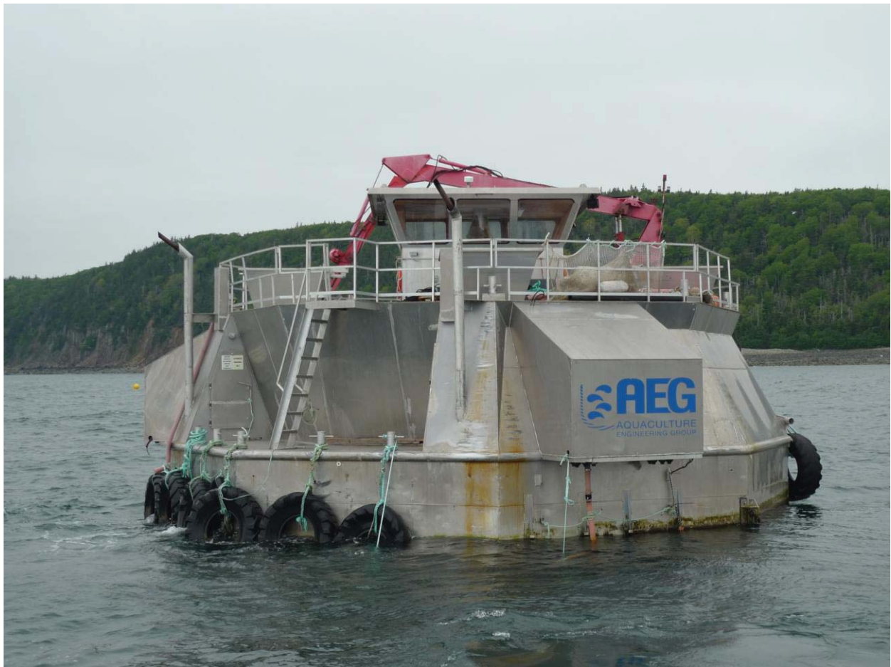
Aquaculture Engineering Group 100 MT auto feed buoy will be fitted with a Dynamic Positioning System for the Initial Demonstration System
